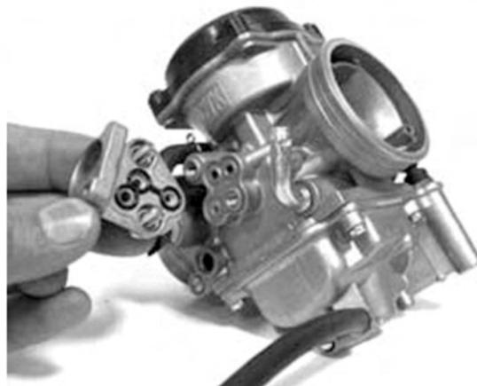
Remove the clamp and the cap with the mem-
