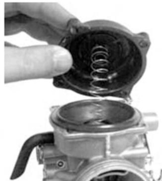
Remove the vacuum valve with the membrane.
