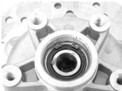
Using the specific tool, remove the ball bearing.
