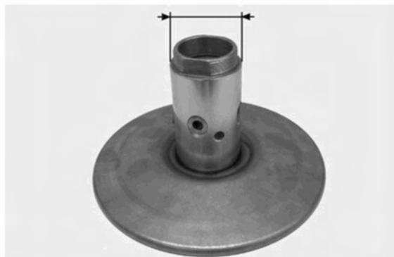
**Inspecting the driven sliding half-pulley**
