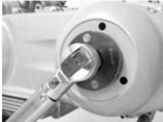
**Specific tooling****020423Y driven pulley stop key****Locking torques (N\*m)****Cover screws 11 ÷ 13 Driven pulley axis (°) 54 ÷ 60**
