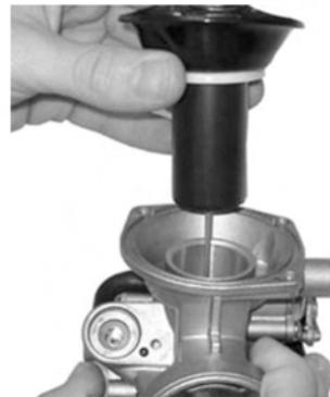
Loosen the coupling by 1/8 turn and remove it, remove the spring and the vacuum valve pin.
