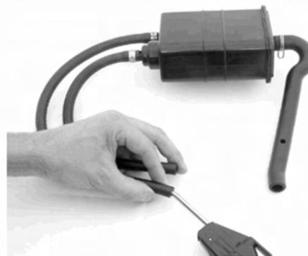
If abnormal noise, clogging or carbon losses are noticed, replace the Canister.
